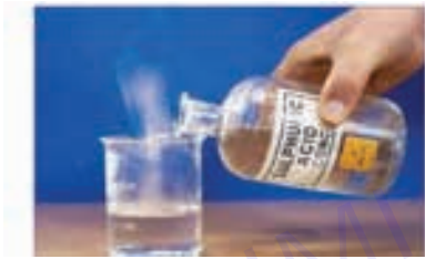
ADD SULFURIC ACID INTO DISTILLED WATER PREPARATION OF ELECTROLYTE
