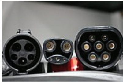
IEC Type 1/SAE J1772 inlet (left); NACS (center); IEC Type 2 connector outlet (right)
