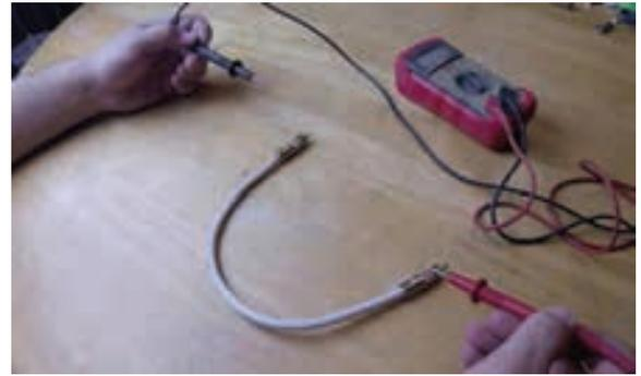
This tracing and beeping will work even if the other end of the coaxial cable is attached to a wall outlet.
