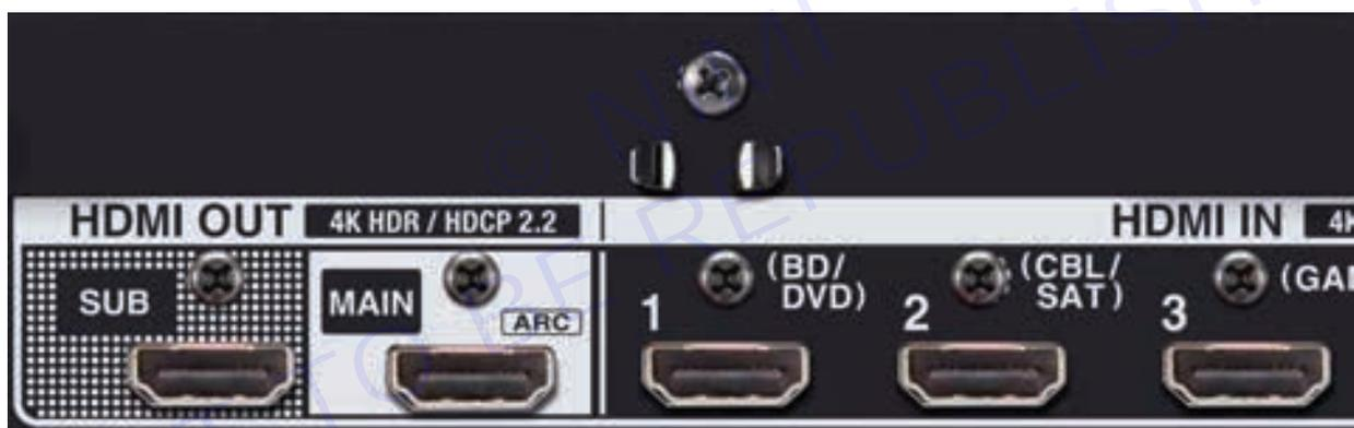
HDMI is the most important connection on modern home theater receivers. (Receivers may also be referred to as AV receivers or surround sound receivers.) It is where you connect HD and 4K source devices, including Blu-ray and Ultra HD Blu-ray Disc players, cable and satellite boxes, media streamers, and game consoles.
