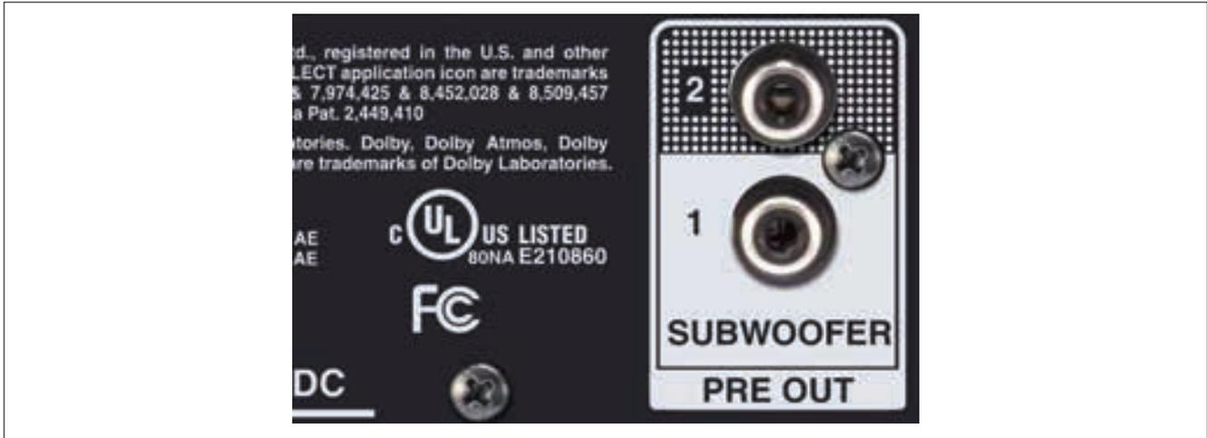
Another type of speaker that needs to be connected to a home theater receiver is a subwoofer. The subwoofer doesn't connect to the terminals provided for the other speakers. Instead, the subwoofer connects to an RCA-type connection that is labeled as Subwoofer, Subwoofer Preamp, or LFE (Low-Frequency Effects) output.
