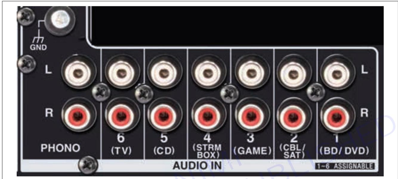
Most audio is available digitally. Still, many devices either use analog exclusively (such as vinyl record turntables, audio cassette decks, and VCRs) or provide it as an alternate audio connection option (using RCA style jacks and cables) on devices such as TVs, cable and satellite boxes, and DVD and Blu-ray Disc players.
