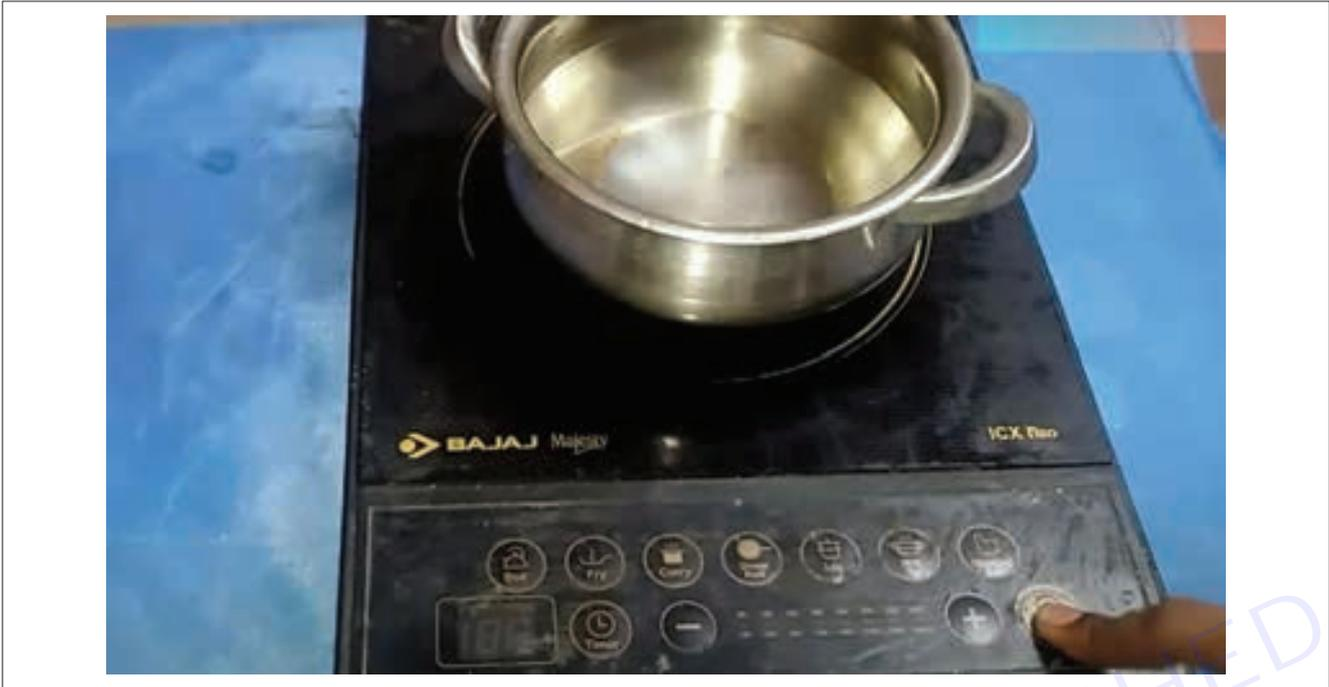
This is not a major complication and is easily solvable. The appliance is equipped with an infrared sensor. It shuts off automatically when no cookware is detected for a few seconds. If your sensor is turned off, it could be because the cookware is not in the centre of the cooking zone. Due to this, it does not get detected. Place it back right. Still not working? Please turn off the power for a few seconds and then switch it on. This can help your appliance reset.
