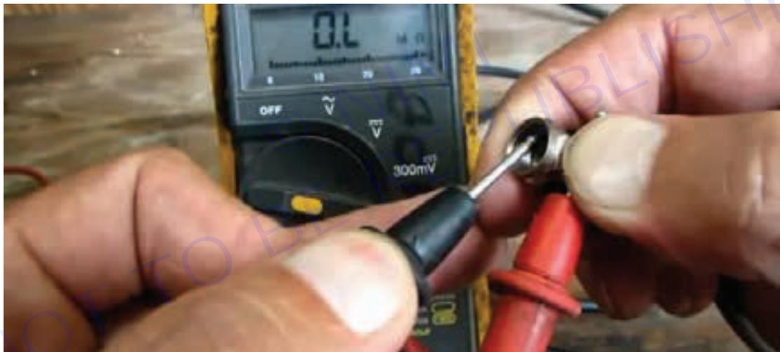
When you attach the tip of your coaxial cable to an external source, touch one probe of the multimeter to where it meets a metallic part. Touch the other probe of the multimeter to where it meets the center wire or core. You're looking for a readout close to zero ohms/
