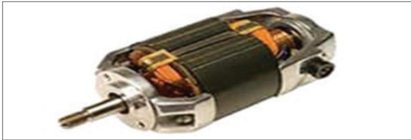
A universal motor is a type of electric motor that can be powered by either AC or DC power and uses an electromagnet as its stator to generate a magnetic field. It is a commutated series wound motor, with the stator field coils connected in series with the rotor windings through a commutator. The universal motor is structurally very similar to a DC series motor but slightly modified to operate with AC power.
