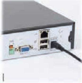
Connect the DVR power supply (marked For DVR use only). Do Not connected it to mains power at this stage.
