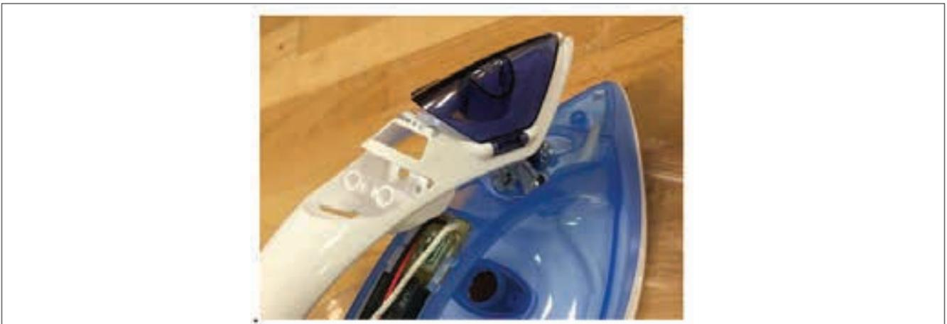
**STEP 10: Circuit Board Removal.**
