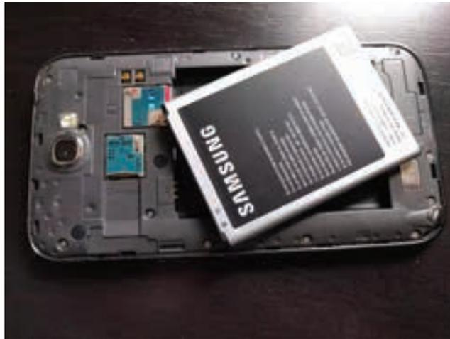
**WARNING:** Don't touch the battery or any components on the device with your fingers. Instead, use a piece of plastic, such as a guitar pick, to pop the battery out. Some devices include a battery lock or switch that you must press to pop it out.
