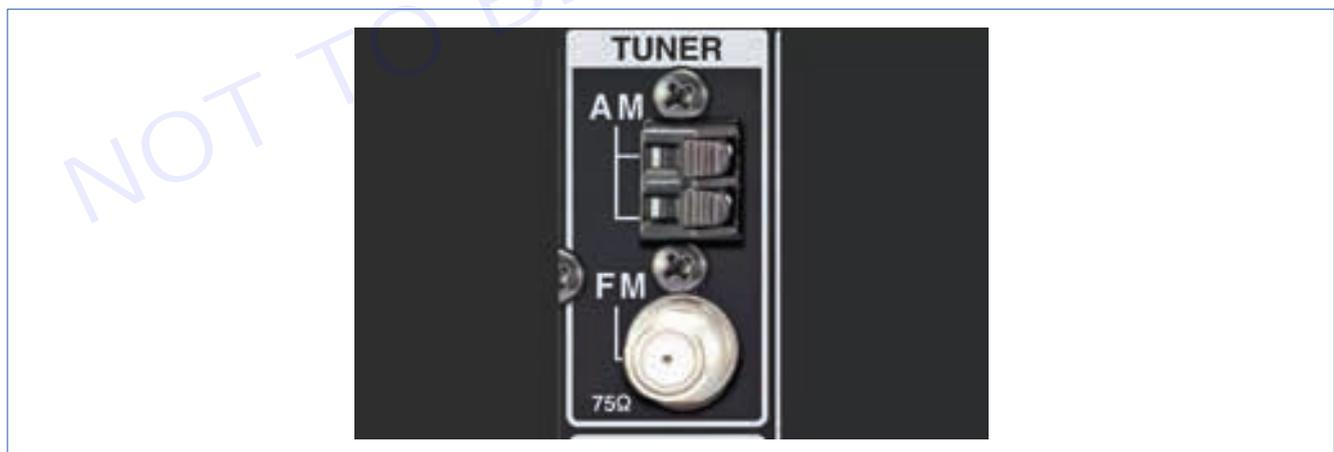
Another audio source included in home theater receivers is radio reception. Most home theater receivers provide connections for AM and FM antennas. However, some home theater receivers only provide FM antenna connections as these receivers may not include an AM tuner.
