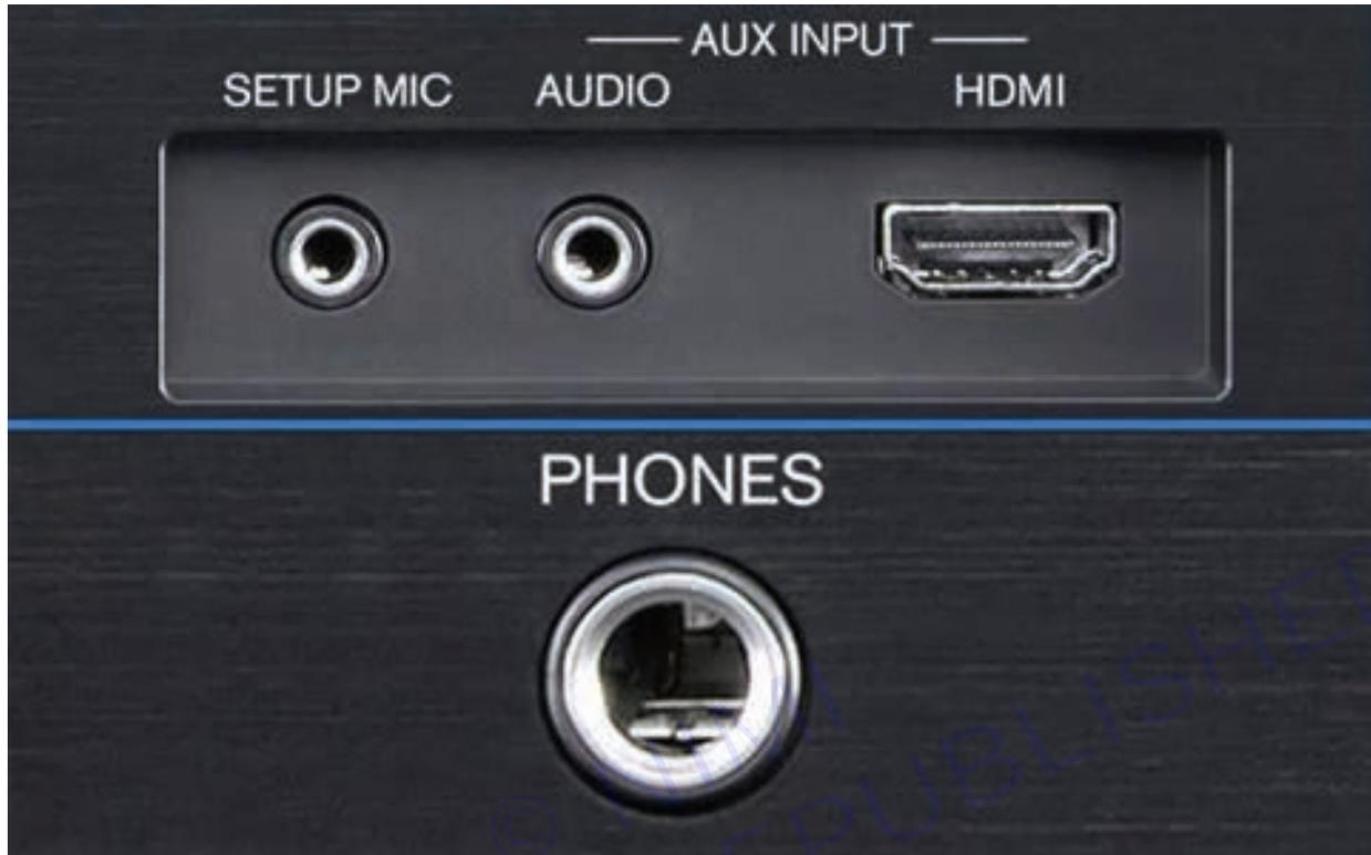
In addition to the connections on the rear panel, many home theater receivers have connections on the front panel. On some home theater receivers, these may be hidden by a flip-down door.
