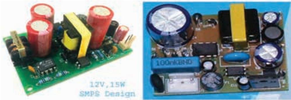
**Note:** Instructor may guide the students to identify the major sections and components of SMPS unit – namely EMI filter, Input fuse, Electrolytic Capacitors, Polyester Capacitors, Thermistor, MOV, Rectifier, Switching MOSFET, SCR, driver IC, PWM IC, driver transistor, Switching Transformer and its pin configuration, Inductor filter, EMI filter, Optocoupler etc.
