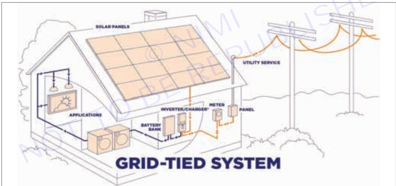
Grid-tied pv inverters connect your home and supplement the electrical grid in case of surplus power generation. The inverter delivers power to your home appliances directly from the solar panel when the solar energy is available for use. It switches back to grid power in case there is insufficient solar energy.
