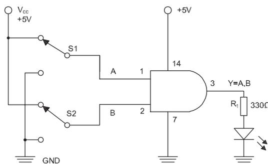
CONSTRUCTION OF AND GATE USING IC 7408
