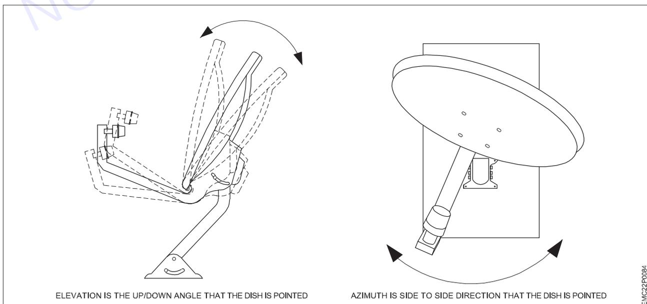
Fig shows - Setting of Azimuth/Elevation Angle for intercepting/collecting satellite signals.
