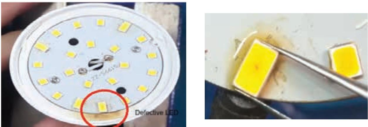
To verify the faulty LED, short the doubtful LEDs one by one with a tweezer or wires as shown in Fig 9. When Power is ON, good LED glows. Faulty LED does not glow. Replace that LED with new one or bypass it as shown in Fig 10.
