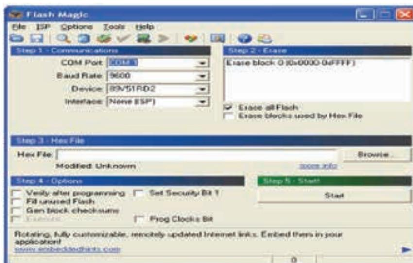
23 Here you have to select the COM number as per Step 1 i.e. shown in above fig, for that you have to select the device manager – Ports (COM & LPT) - USB Serial port (COM 1), it varies kit to kit.
