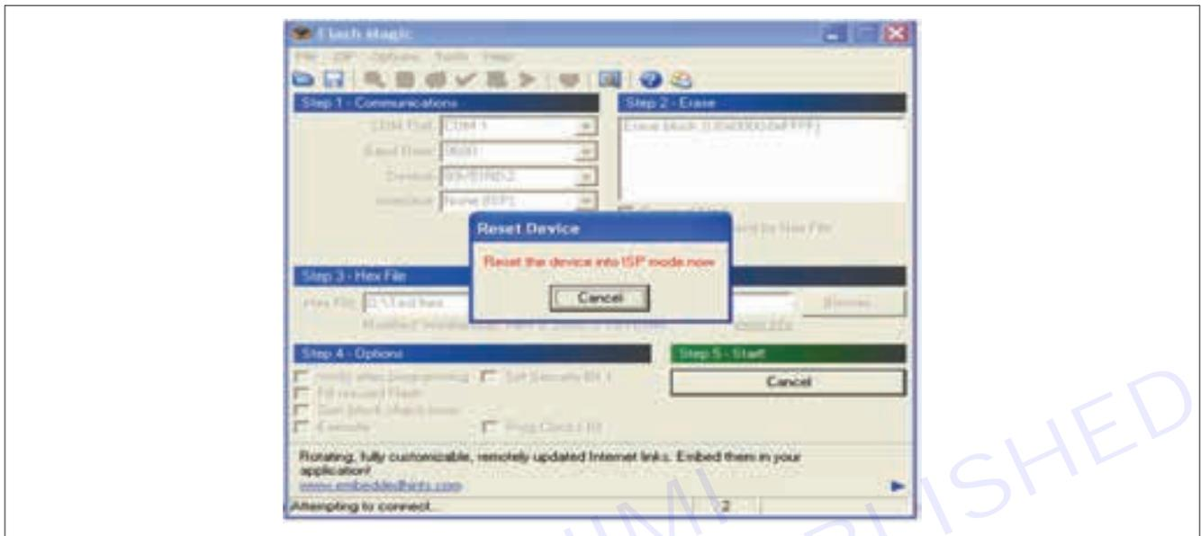
27 Start the program by pressing start button of step 5 as shown in the above Fig
