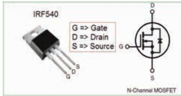
To test a MOSFET, assume an N-channel MOSFET. For example, IRF 540 has 3 terminals namely Gate, drain and Source. Set the DMM in diode mode.
