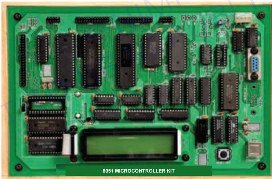
**Note:** The instructor should guide the trainees in identifying and locating various Integrated Circuits (ICs) within the microcontroller kit. It is also important to provide detailed instructions and information regarding the types, functions, and placements of the ICs present in the kit.
