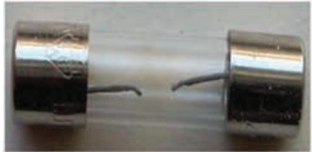
6 Look at the fuse carefully if any dark or metallic smear is seen inside the glass as shown in Fig 8.
