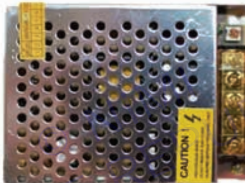
Switch Mode Power Supply power supply
