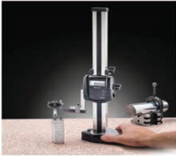
Checking parallelism and perpendicularity
