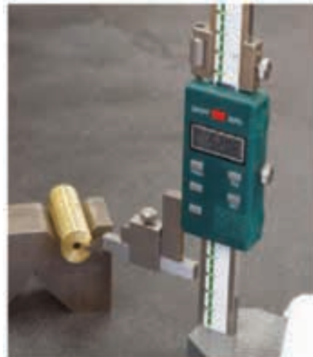
Transferring reference heights for marking or machining operations
