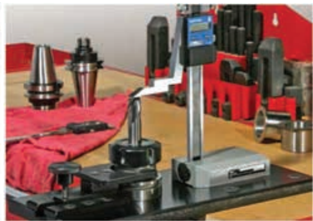
Setting tool heights on machines like milling machines or drill presses
