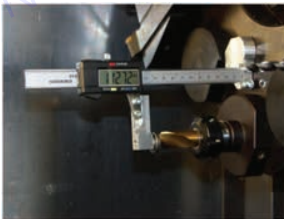
Setting tool heights on machines like milling machines or drill presses
