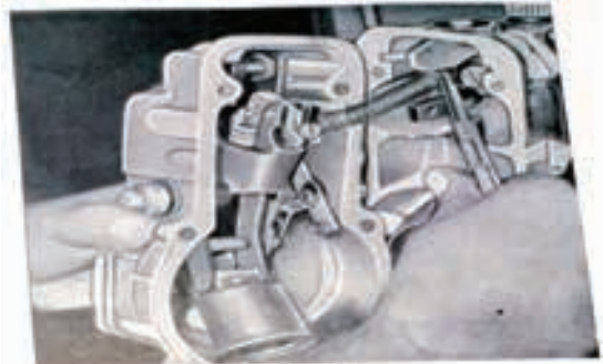
Unhooking the starting spring
