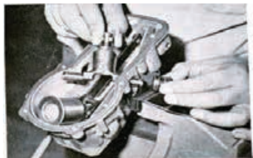
Removing the swivelling lever
